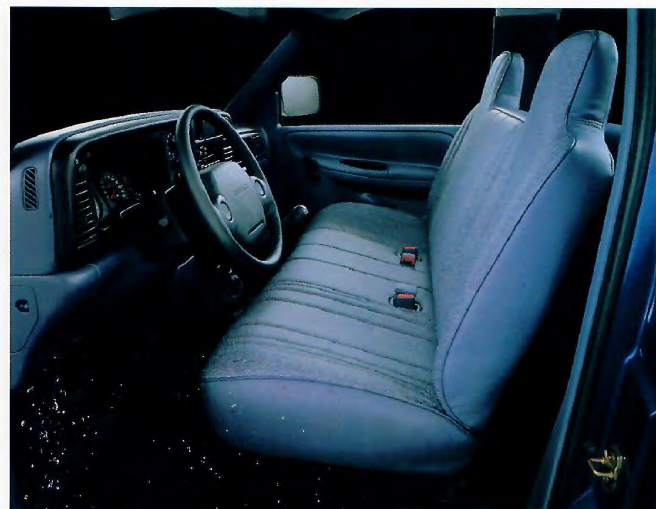
♦ The RAM WS and LT regular cab interior, shown in Slate Blue, includes a solid-back bench seat with tough, cloth-backed Fusion vinyl fabric featuring a pebbled texture for greater comfort. (Also available in deluxe cloth.) The hinged seatback folds forward for access to behind-seat storage.
